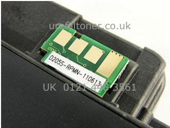
Peel backing off replacement chip and stick firmly into position on top of original chip as shown
