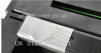
Clean surfaces and apply grey duct tape (Gaffa tape) patch
